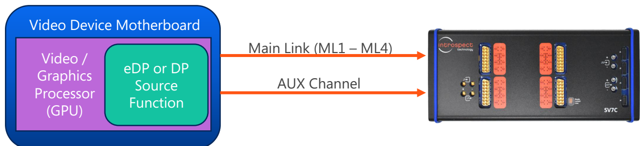
The SV7C-eDP Analyzer Connected to a DisplayPort System
