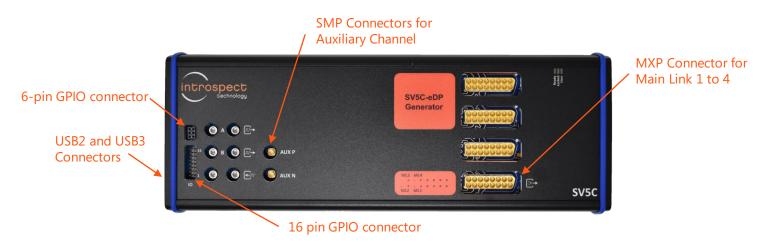
The SV5C-eDP Generator's lanes (main link 1 to 4) are contained on a single MXP connector.
