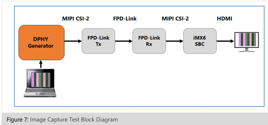
Figure 7: Image Capture Test Block Diagram
