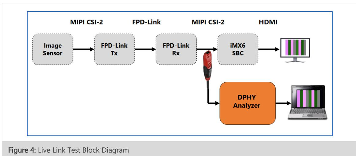
Figure 4: Live Link Test Block Diagram
