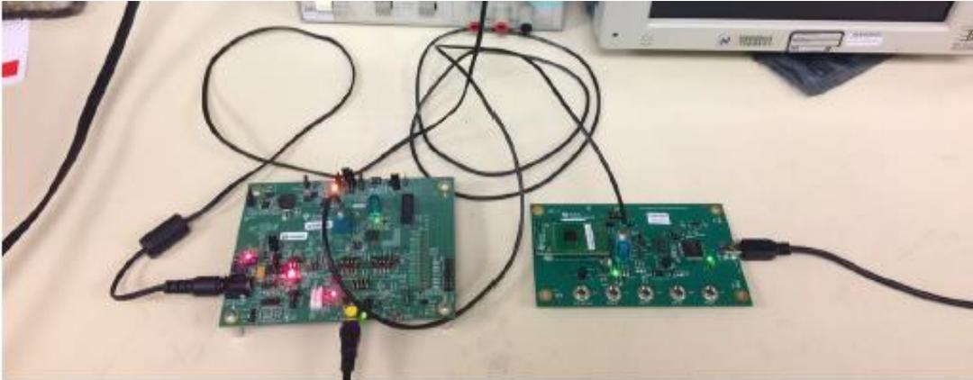
Figure 3: FPD-Link III sub-system under test (DUT)
