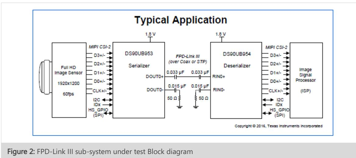
Figure 2: FPD-Link III sub-system under test Block diagram
