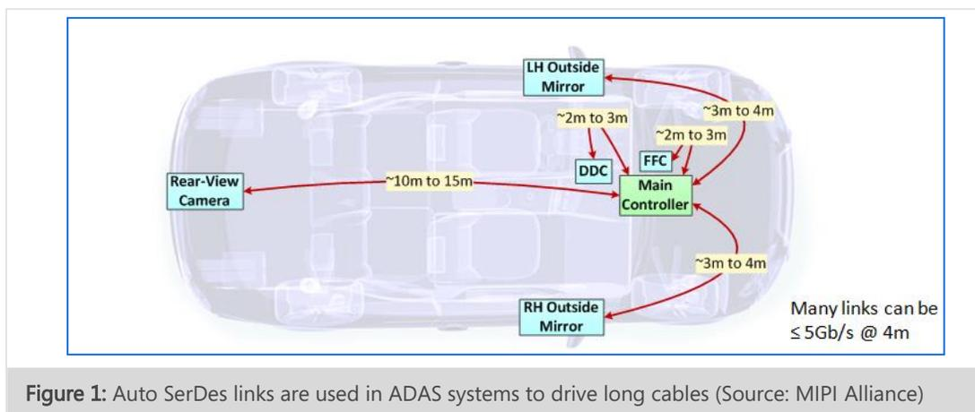
**Figure 1:** Auto SerDes links are used in ADAS systems to drive long cables (Source: MIPI Alliance)
