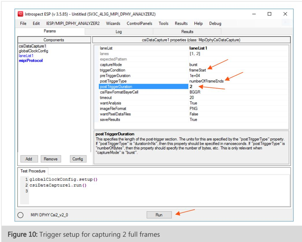
Figure 10: Trigger setup for capturing 2 full frames
