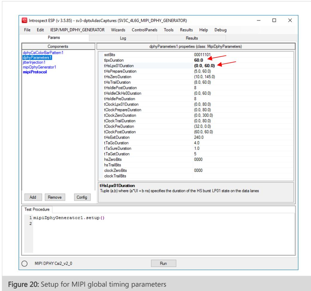
Figure 20: Setup for MIPI global timing parameters
