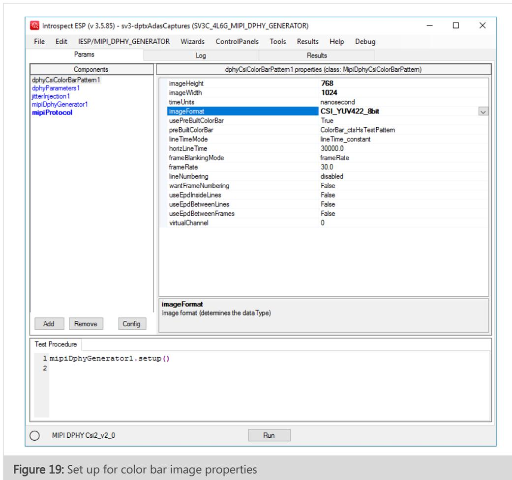
Figure 19: Set up for color bar image properties
