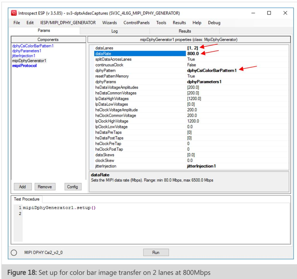
Figure 18: Set up for color bar image transfer on 2 lanes at 800Mbps
