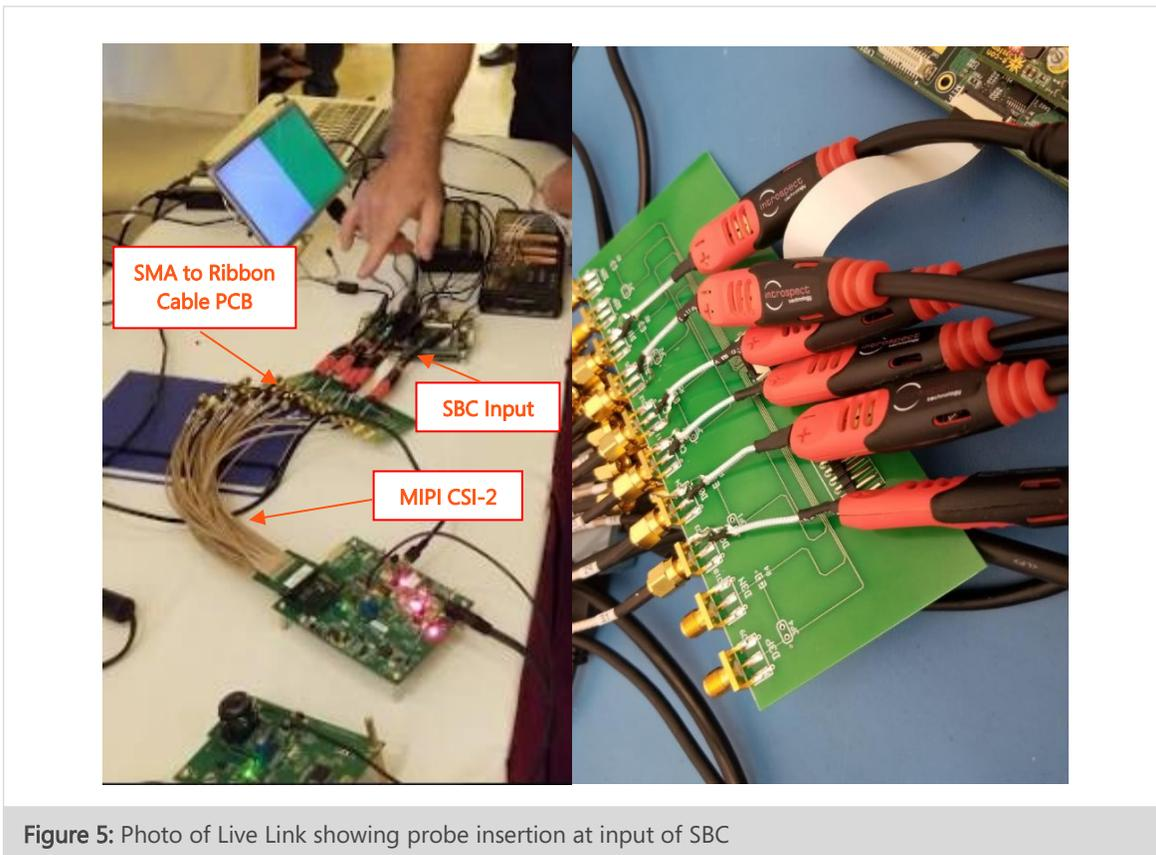
Figure 5: Photo of Live Link showing probe insertion at input of SBC
