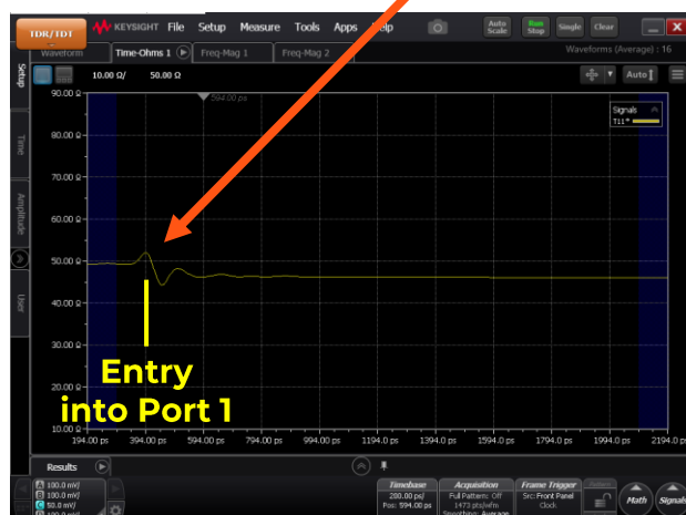
Figure 2: T11 (left) and S11 (right) performance of the LP5-315-P interposer.
