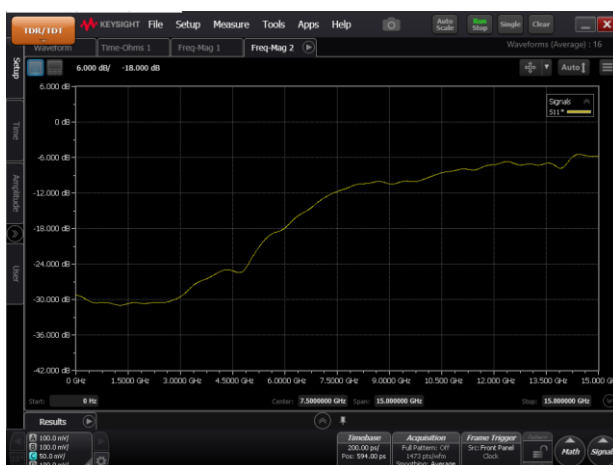
Figure 2: T11 (left) and S11 (right) performance of the LP5-315-P interposer.
