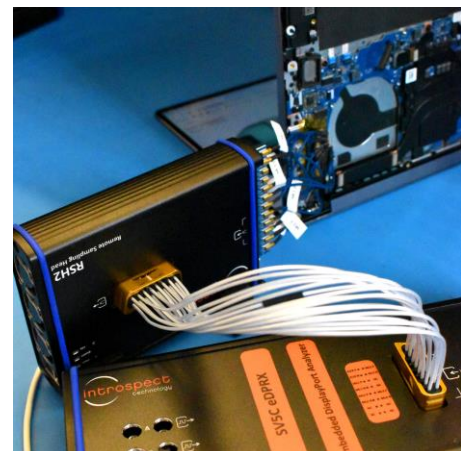
Probing an Embedded DisplayPort application with the SV5C-eDP Analyzer and RSH2 Remote Sampling Head
