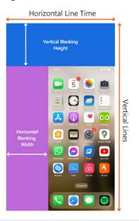
Protocol analyzer capture of an eDP mobile screen
