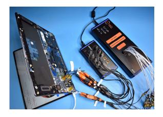
Probing a DisplayPort application with the SV5C-eDP Analyzer
