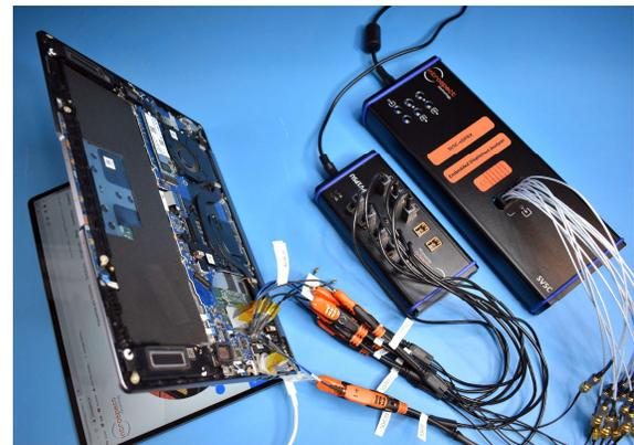
Probing a DisplayPort application with the SV5C-eDP Analyzer
