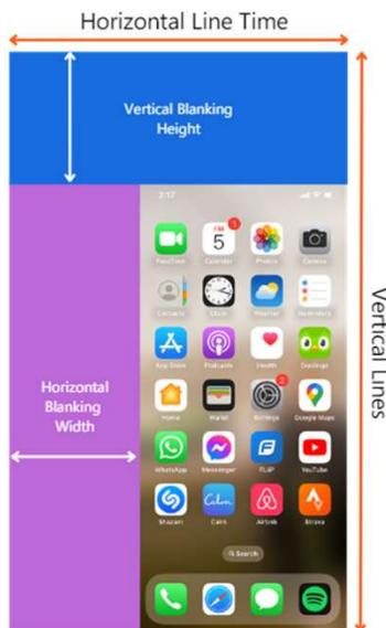
Protocol analyzer capture of an eDP mobile screen
