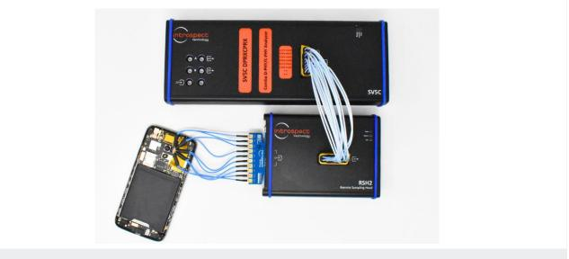
The RSH2 Remote Sampling Head and the SV5C-DPRXCPRX D-PHY and C-PHY Analyzer Probing a Smartphone Camera
