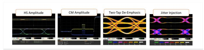
SV3C-DPTX waveforms illustrating voltage, timing, and signal integrity controls required for receiver testing
