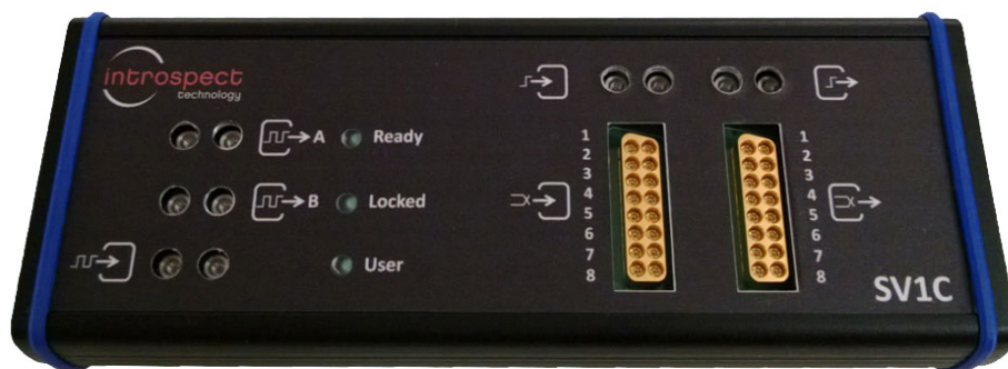
Figure 2 SV1C Personalized SerDes Tester used for jitter transfer measurement
